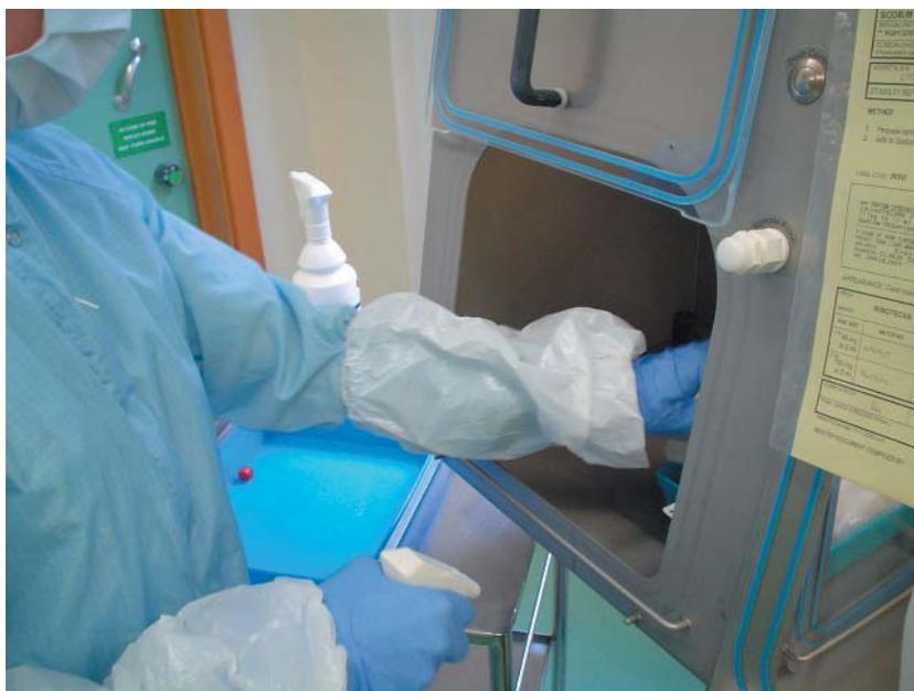
**Figure 3** Prepared product being removed from isolator about to be sprayed with alcohol.
