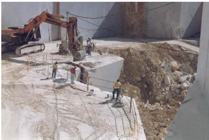
**Figure 2** Overturning of the bench with an excavator.
