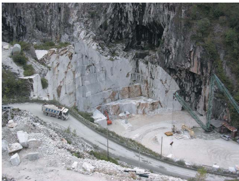
Figure 3 Quarry site: rubble transport (a derrick and an excavator are visible).
