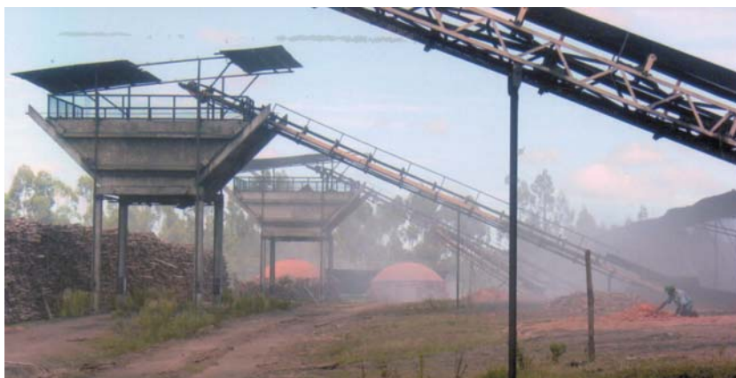
Figure 7 Silos that enable direct charcoal truck loading.
