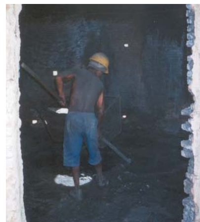
Figure 4 Taking charcoal out of a kiln.
