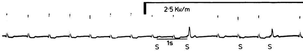
Fig 1 Reversion of pacemaker to interference mode when the patient (case 1) stood with raised arms in substation where an electrical field of 2.5 kV/m was encountered and a corporeal current of 41  $\mu$ A was induced. (S = pacing stimulus.)
