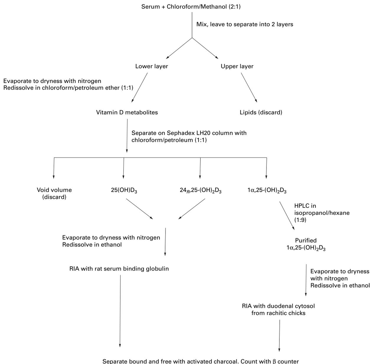
Figure 1 Procedures in the analysis of vitamin D<sub>3</sub> metabolites.
